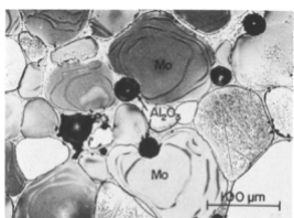
Figure 4 Typical etch boundaries within growing molybdenum grains in contact with Al 2 O 3 particles in a 94.4Mo-5Ni-0.6Al 2 O 3 alloy cyclically sintered at 1460°C with four holding times (1 + 1 + 1 + 1 h).
